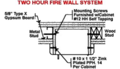
waster UL Classified 5/8" Type X gypsum board inserted in the cavity between the two layers. Warnock Hersey has approved the Safeguard Cabinets to be mounted in any face of fire rated. steel or wood stud for up to 2 hour rated walls without affecting its fire rating. The above meets the requirement test ASTM-E119-98 with test report WHI-495-1534. MOUNTING INSTRUCTIONS are supplied with each Safeguard cabinet.
